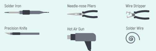
\* These are not included in the DIY Kable Kit. Tools listed represent the best choice for the respective tasks. You can still complete the Kit using alternatives, e.g. a lighter instead of a hot air gun.
