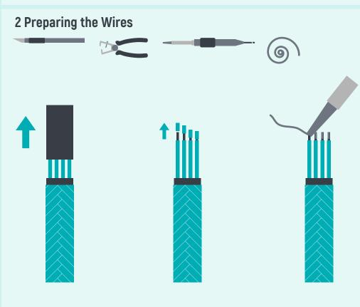
Cable: strip 15mm cable insulation. Wires: strip 5mm wire insulation.
